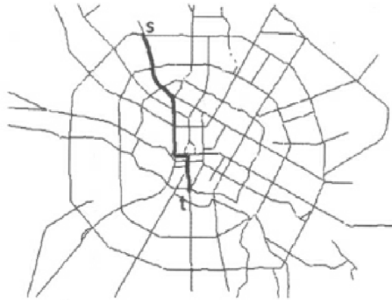
Figure 2. The optimal path obtained by Dijkstra algorithm.
